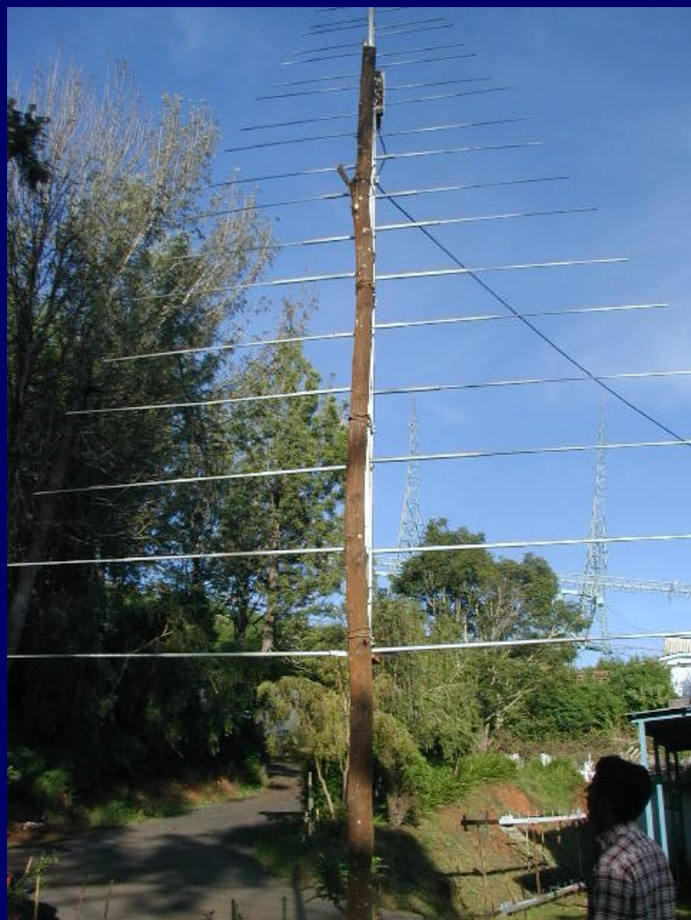
Left: Self built antenna.
